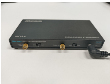
Figure 1 Powered by the standard 12V DC adapter.
