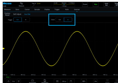
Figure 4 In the Userset interface of the oscilloscope, choose Aux Out--Clock In
