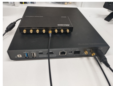
Figure 2 Clock synchronization connection.
